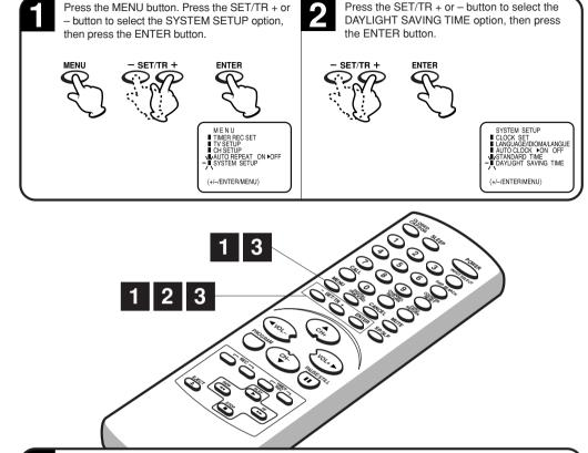
Press the SET/TR + or - button to select one of the options, then press the ENTER button. Press the MENU button until the MENU screen is cleared.
